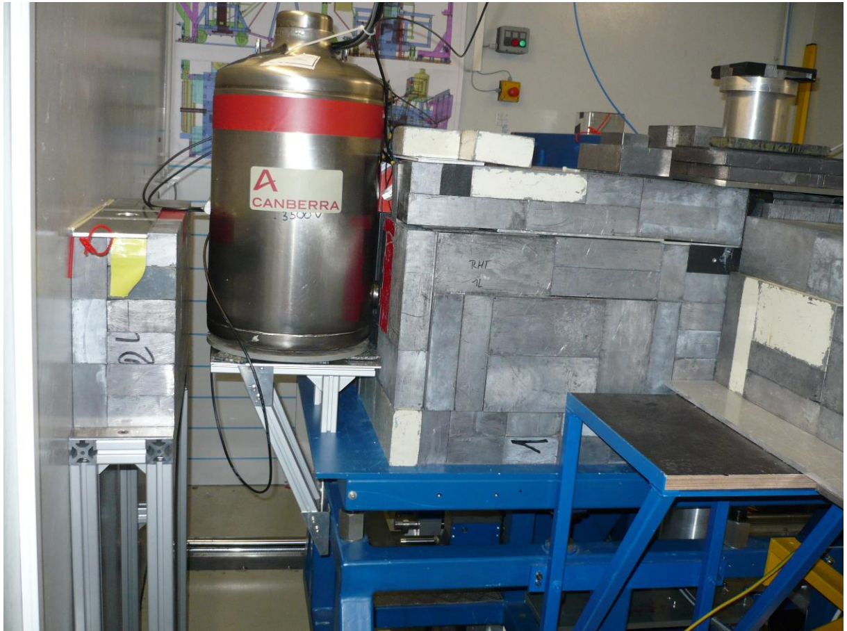
Figure 12. Shielding (cover removed) of the detector system.
