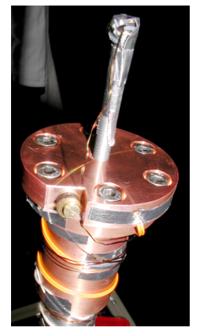
photo: CC-cold head, flange 2nd stage, for testing with an Alu-M6-threaded rod and adhered sample thermometer
