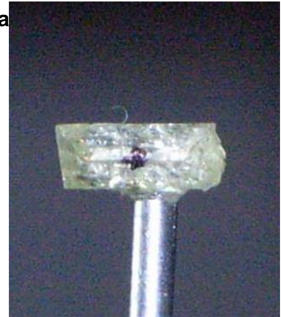
Brazilianite sample on aluminum pin (1mm) for measurement on HEiDi/MLZ
