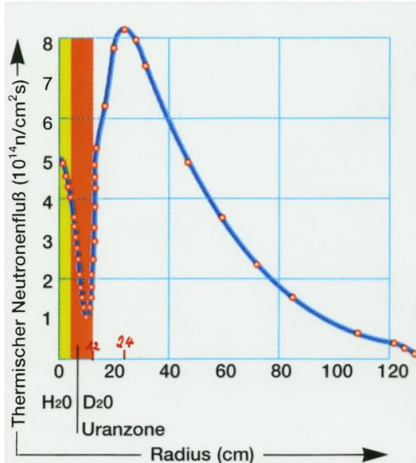
Thermal neutron flux over radius R in the mid-plane of the fuel element.
