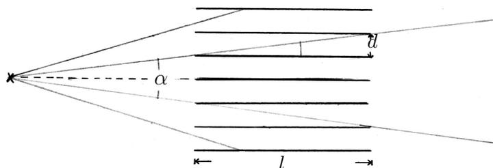
**Figure 12:** Drawing of a Soller collimator. The divergence of the outgoing beam is  $\tan(\alpha/2) = d/l$ , which is in the example ca.  $18^\circ$ . On PANDA the collimation can be chosen between 15 and 80 minutes.
