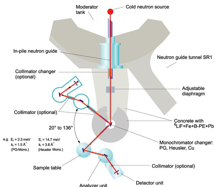
**Figure 11:** Schematic design of a three axis spectrometer.
