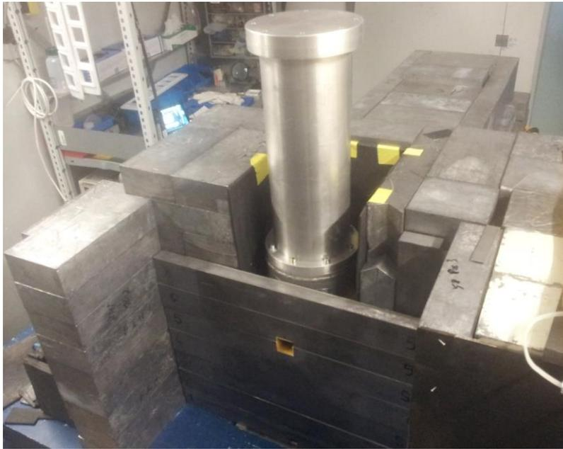
Figure 12. Shielding of the sample chamber.
