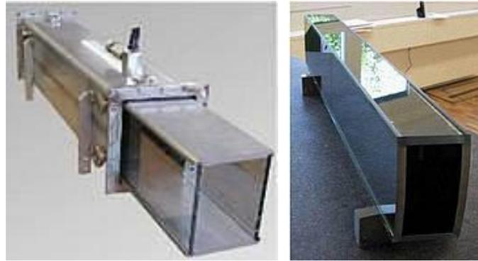
Figure 3. Neutron guides (source: FRM II web page)
