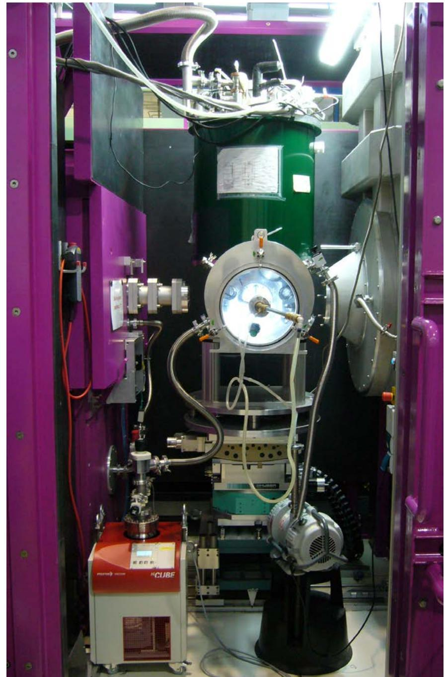
Vacuum vessel for detector to provide lowest possible background
