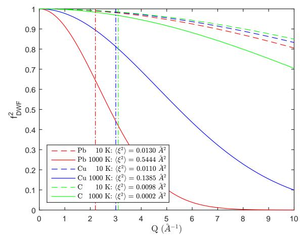
The vertical lines indicate the first allowed Bragg reflexion, which can be used for monochromatizing neutrons. The most useful monochromator material obviously would be diamond. Lead, on the other hand, is quite unsuitable. The reflectivity of copper, which is a commonly used monochromator because it is easy to produce large good quality single crystals, benefits strongly from cooling it down.
