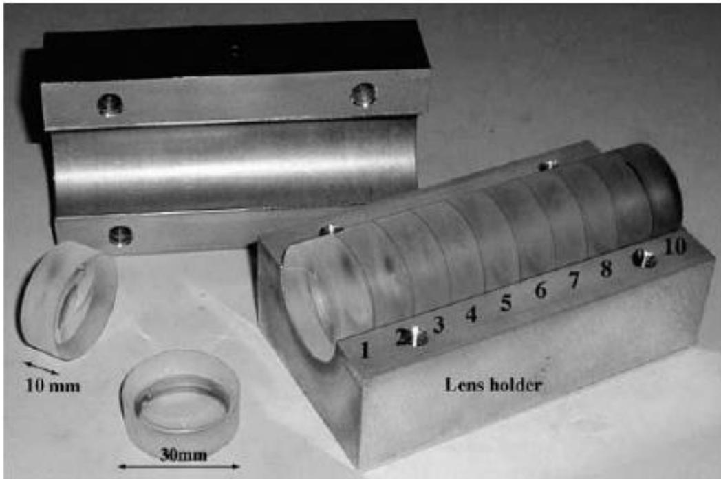
Figure II.1.3.2.5 Biconcave refractive lenses, made from a single crystal of magnesium difluorides ( $\text{MgF}_2$ ), which are aligned in an aluminum holder.
